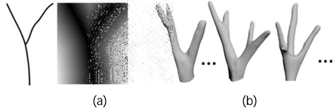
Fig. 4. Cut retrieval: from a simple user sketch (a) we compute a descriptor (a)-right which is used to retrieve a set of best matching cuts from the repository, sorted according to their similarity (b).
